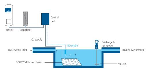
SOLVOX diffusion hoses application. Oxygen transfer via tubular diffusion hoses made of a chemical resistant elastomer rubber material installed on the bottom of the tank.
